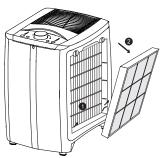
5 Slide the HEPA along the slot and remove it by lifting it outwards
