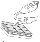
6 Clean or replace the filter with a vacuum cleaner (Pre Filter can be washed with water and dried before
